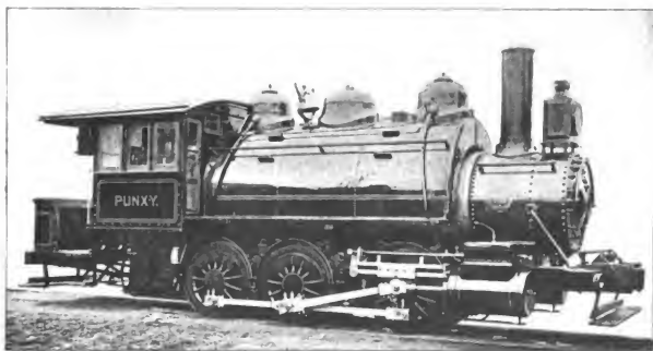
Fig. 14. Six-Wheel (0-6-0) Tank Switching Locomotive. Built by the American Locomotive Co. Cylinders 17 in. x 24 in., Working Steam Pressure 180 lbs. per sq. in., Diameter of Drivers 46 in., Weight on Drivers 96,000 lbs., Total Weight 96,000 lbs.
